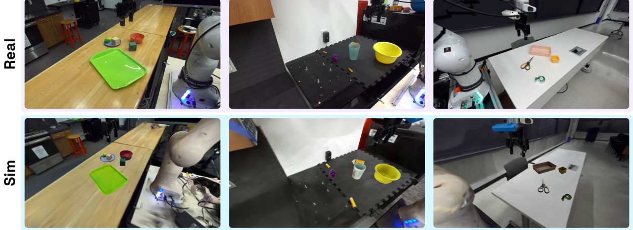
Figure 5 | Evaluation environments. Top: real-world environments, Bottom: POLARIS simulated evaluation replicas. We create high visual fidelity environments utilizing Gaussian Splats for environment reconstruction and TRELLIS for object asset generation.
